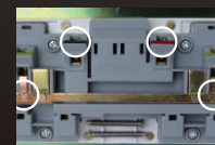
Double earth terminals for safer sockets
